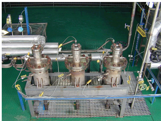
Fig. 6. Pilot plant reactors used to study oxidation of ammonia and decomposition of nitrous oxide.
